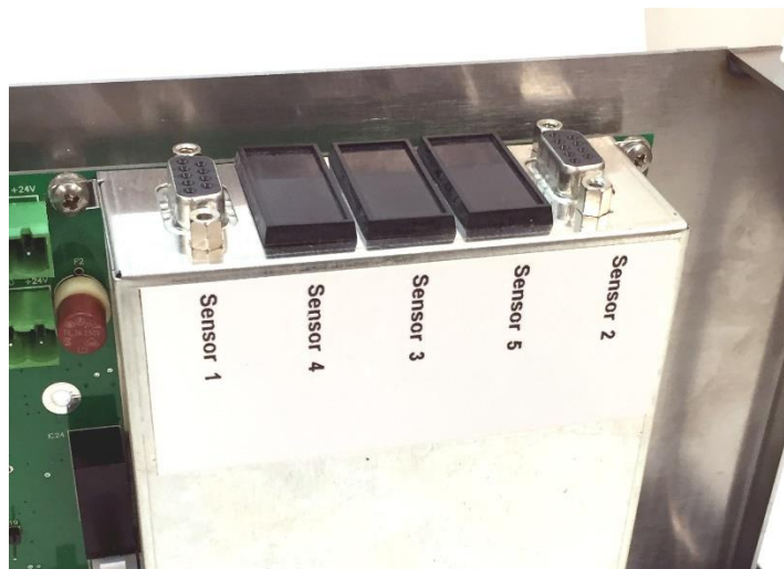
Figure 13 Control board with 2 sensor boards under the EMC enclosure.
