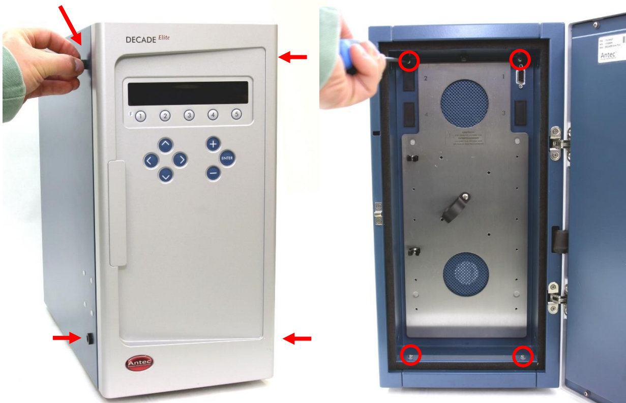
Figure 14 Left: removal of the rubber liners in the inlet/outlet openings in the detector oven compartment. Right: Removing the M3 screws securing the detector cell cabinet.
