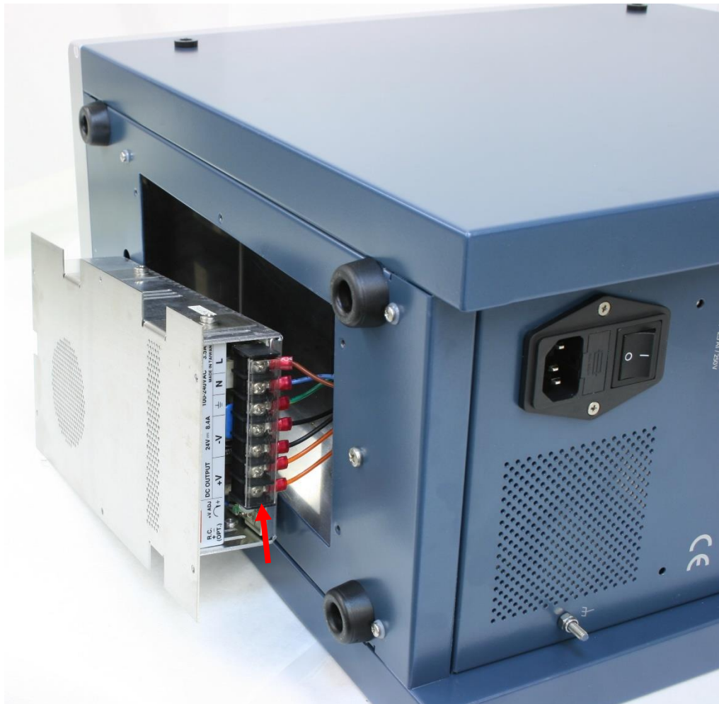
Figure 20. PSU frame with PSU and connected wiring of the primary and secondary power circuitry. Arrow indicates the plastic cover strip.
