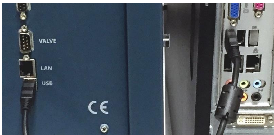
Figure 2 Left: rear panel DECADE Elite with USB cable connected (B type connector). Right: rear panel of the PC with USB cable connected (A type connector).
