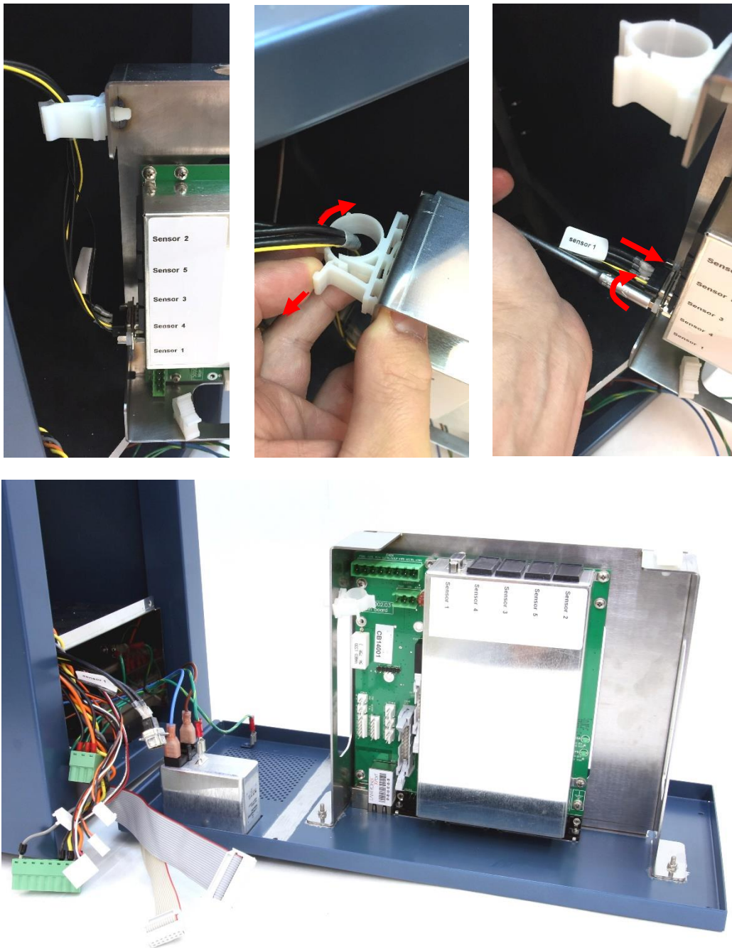
Figure 9 Top-left: Move PCB frame backwards to access the internal cell cable connection on sensor board 1. Top-middle: remove internal cell cable from the cable clamp. Top-right: loosen the 2 hex screws fixing the internal cell cable to the sensor board connector and disconnect the cable. Bottom: The back panel with PCB frame can now be moved out of the electronics compartment completely and can be placed on the table.
