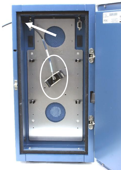
Figure 5 Take out flow cell and place temperature sensor within white circle and close the door. Insert the temperature probe via the tubing hole (arrow) and close the door.
